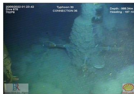
Figure 8: Real-time images showing gas flow at wellhead (LHS), High intensity SONAR reading confirming gas flow from deeper depth interval (RHS) and Real-time image showing low flow at wellhead while drilling Agnob 71 well. The flow diminished after circa 5 hours of flow (Bottom).
